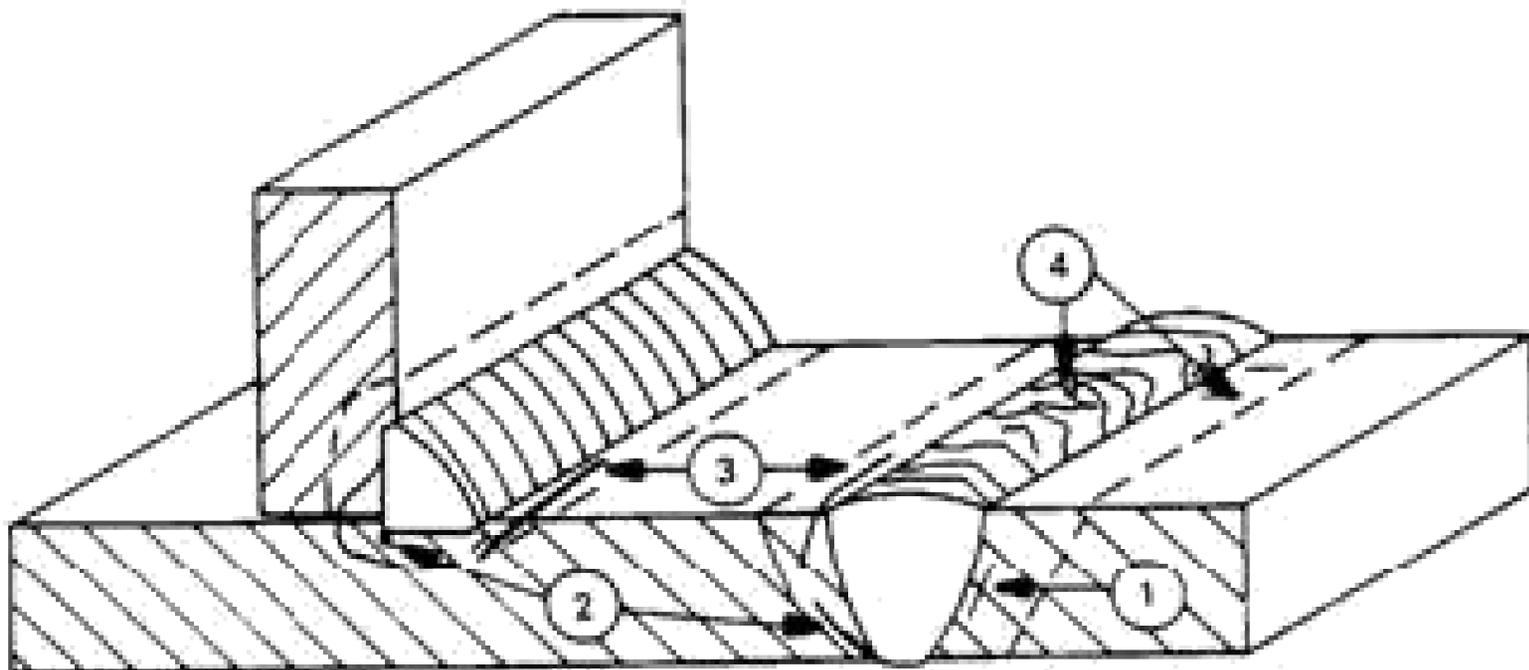
1. trinca sob cordão (underbead crack)
