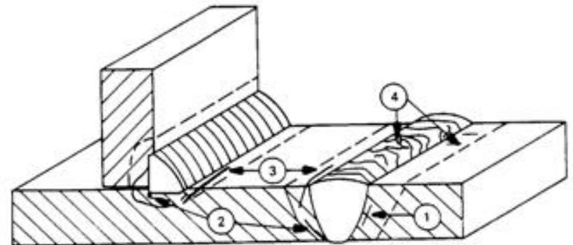
1. trinca sob cordão (underbead crack)
